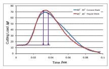
The new Concave Cobalt scissors will cut hair very well with less effort, because the cutting load is lower than existing scissors.
